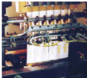
A Model 2012 12" (305mm) Standard Air Knife opens mustard packets prior to fill.
